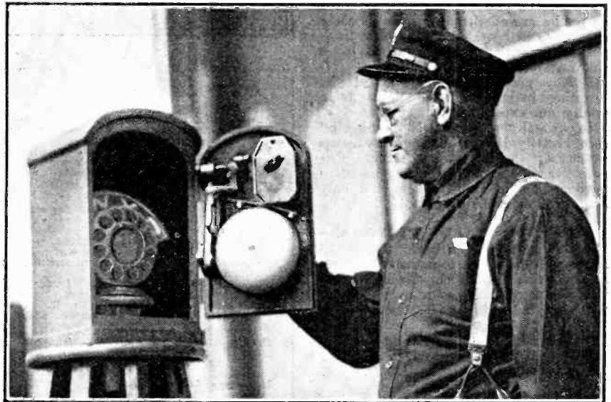
WIRELESS FIRE ALARM. An interesting device now being tested by the New York Harbour Fire Department. By its use firemen on shore are able to keep in telephonic communication with their colleagues in the harbour and give notification of fires.
