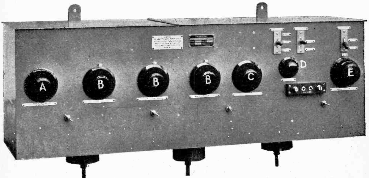
The type R.g.18 receiver, which covers a single waveband. A, aerial tuning condenser; B, secondary and H.F. tuning condensers; C, gang control knob; D, volume control rheostat; E, local oscillator condenser.
