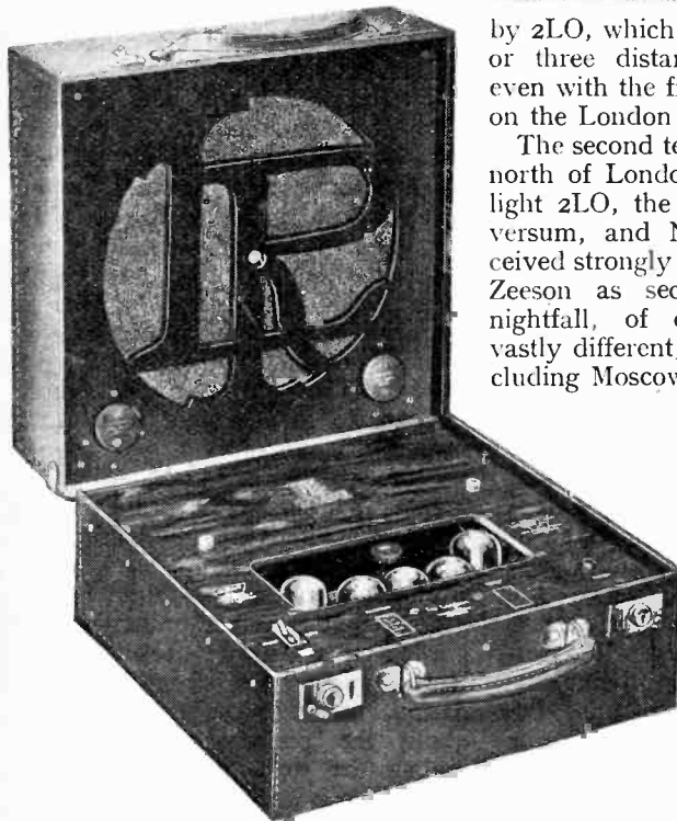
The Langham Transatlantic Portable which has drum-type tuning control and dial.
